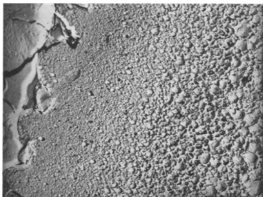
Figure 5 Region of final failure. Crack growth from right to left \times 920 .
